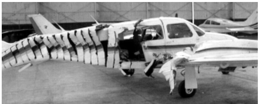
An Aussie doctor had a dead battery so, with ignition on, a little choke, and brakes OFF, he swung the prop. The engine started and the plane taxied at high speed, its titanium blade spinning at 85% of max. RPM. It wiped out about six light aircraft belonging to a local flying club before coming to a stop after slicing up this twin.
